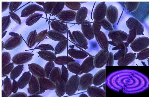
FIGURE 5 Example for food treatment by nonthermal atmospheric pressure plasma. Dill ( Anethum graveolens ) seeds treated with dielectric barrier discharge (DBD). Small photo: DBD with plasma turned on, ring-shaped electrode configuration. Taken from Ref. [85]. Reproduced with kind permission by the authors and Biblioteca Horticultura
